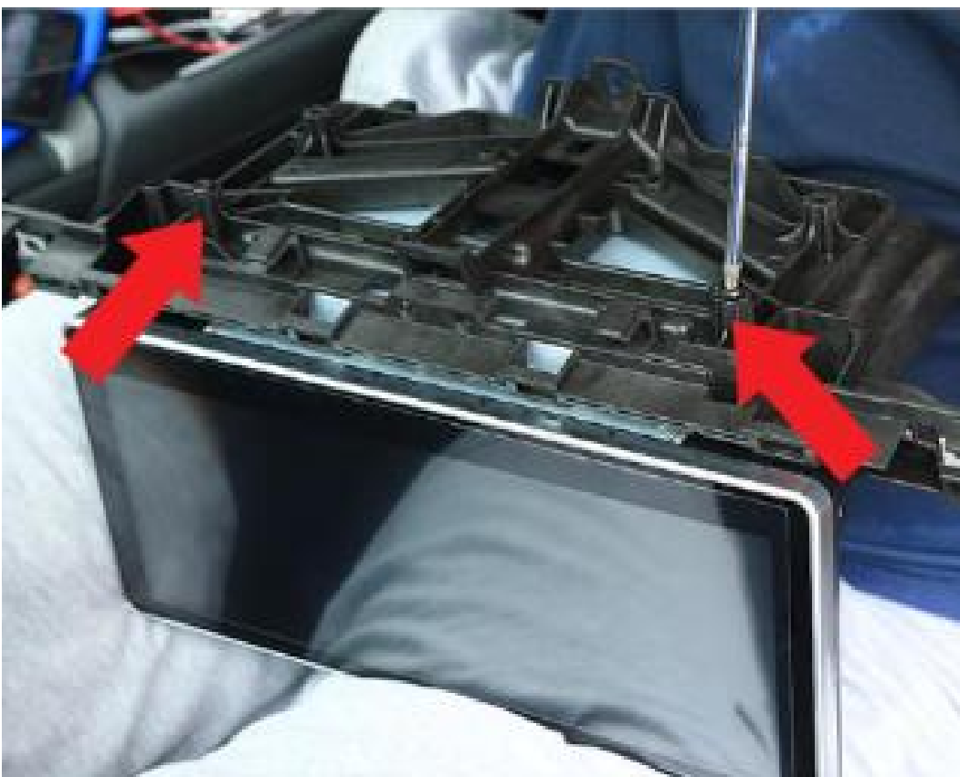
19. Install the provided main harness by routing the white main connector to the LCD screen area
