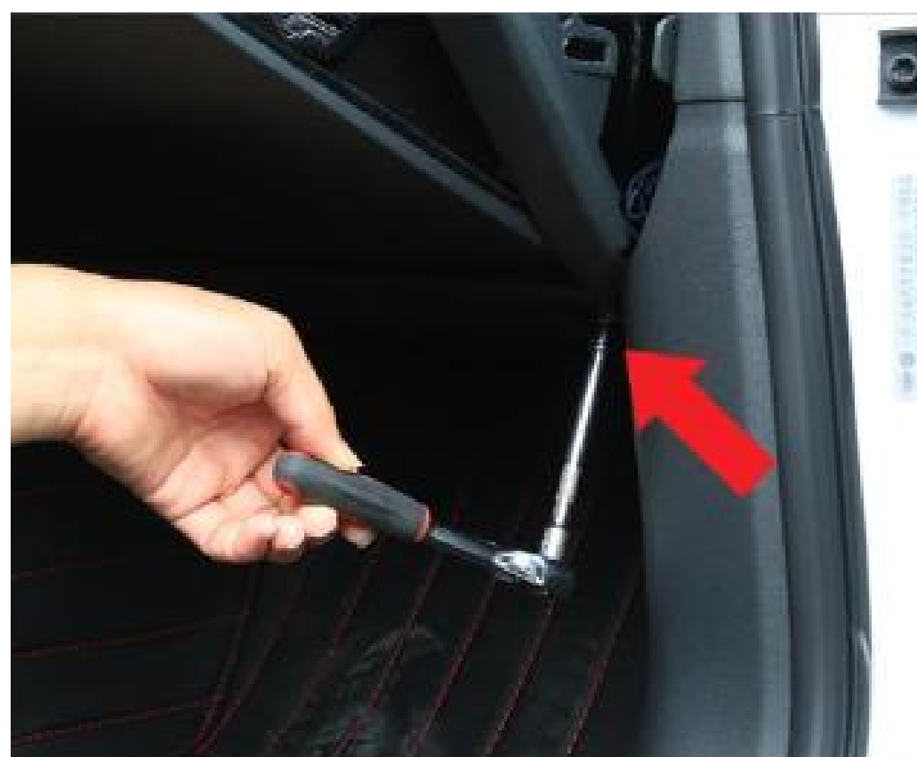
10. Remove the two screws located at the bottom of the glove box and then detach the glove box by pulling it downward.
