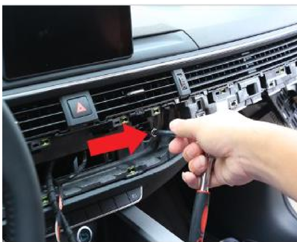
14. Unscrew the four 8mm hex screws inside.
