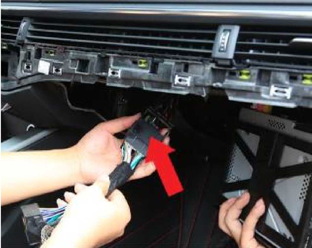
19. Install the provided main harness by routing the white main connector to the LCD screen area
