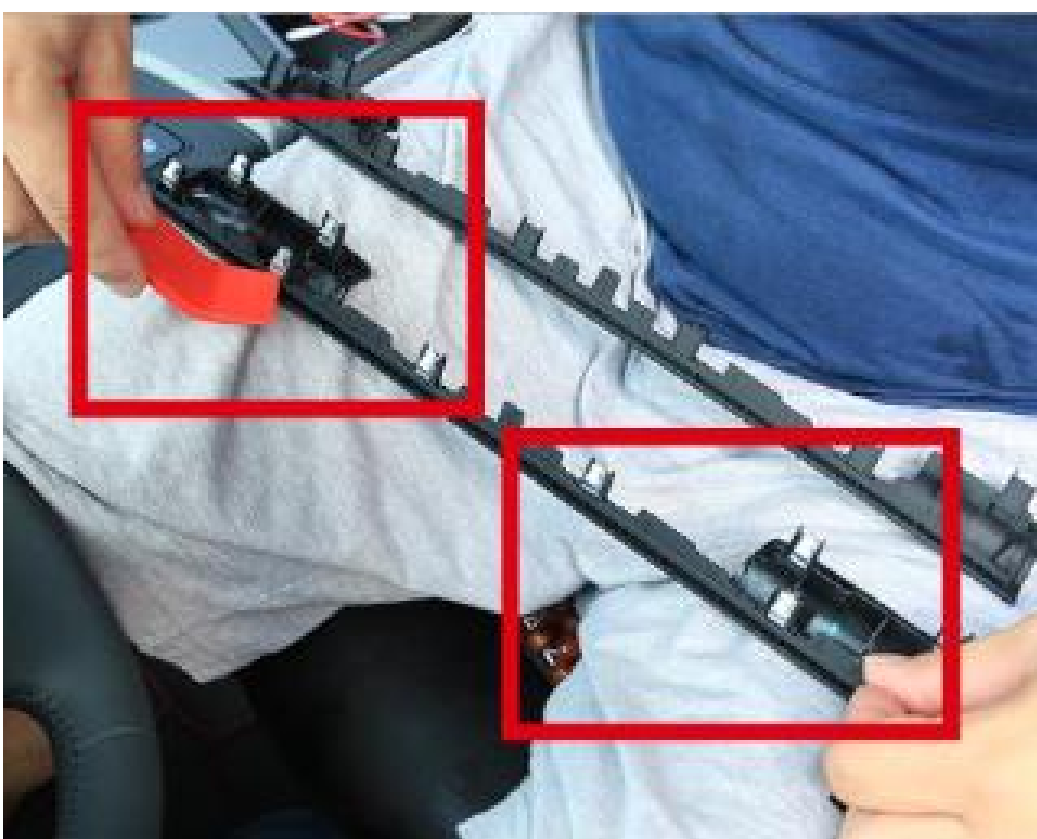
23. Transfer all the original metal clips to the new lower screen trim provided in the kit and then install the trim
