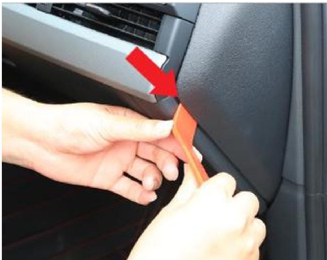
7. Remove the passenger side fuse panel cover using a prying tool
