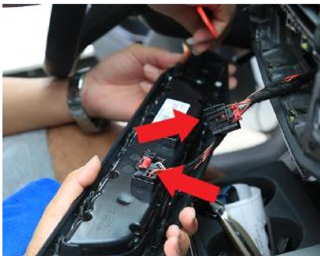
13. Unmount the climate control and unplug all the connectors.
