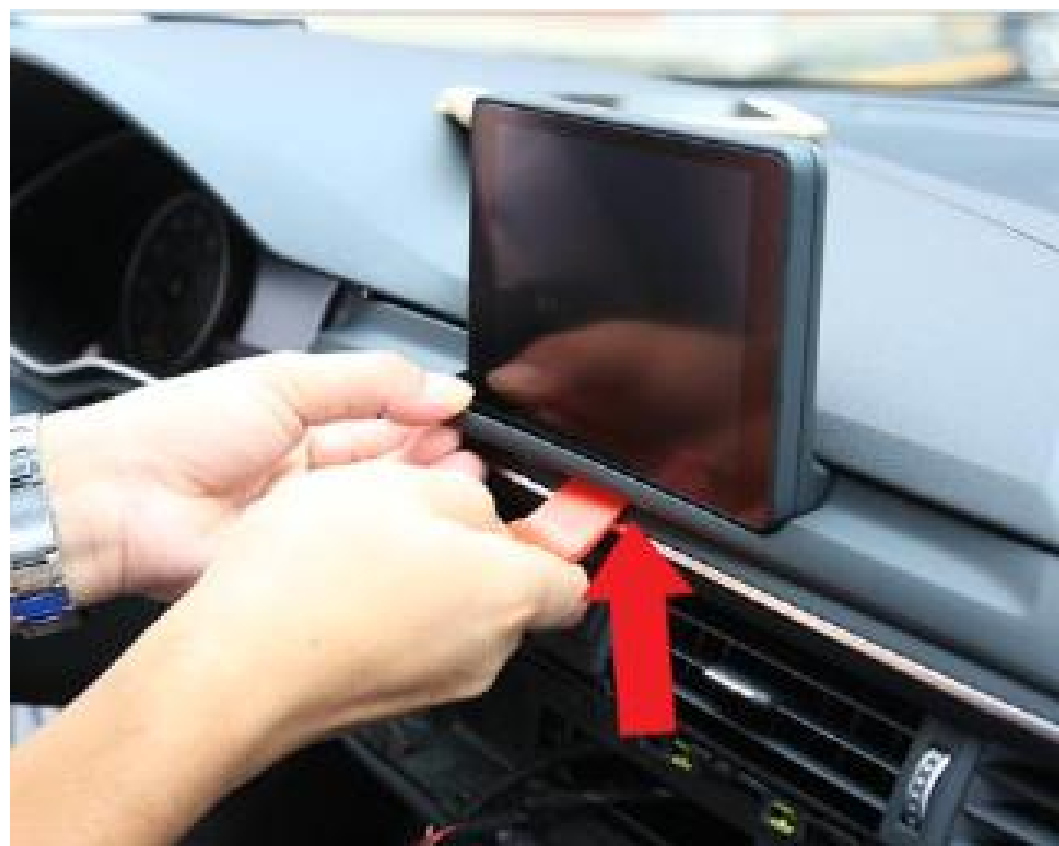
13. Unmount the climate control and unplug all the connectors.
