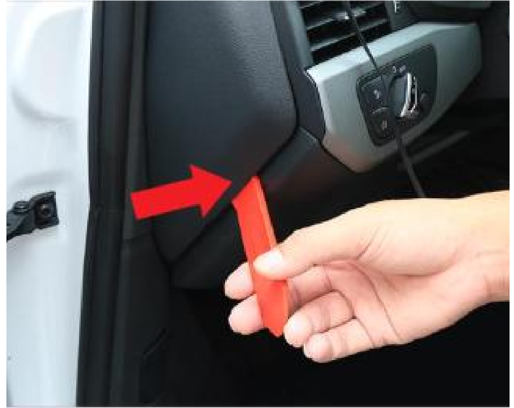
2. Using a prying tool, take off the cover of the driver-side fuse panel.
