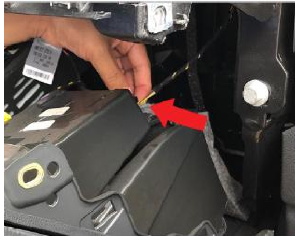
8. Unplug removable connectors from the glove box.
