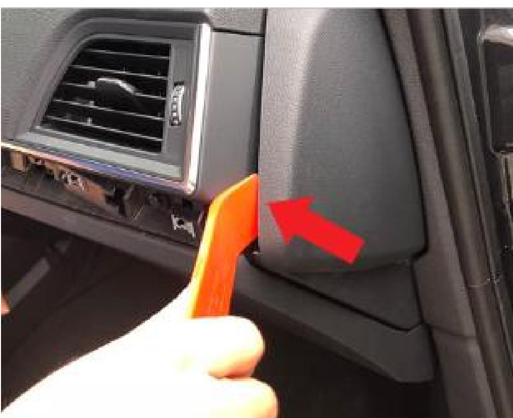
5. Remove the passenger side fuse panel cover.
