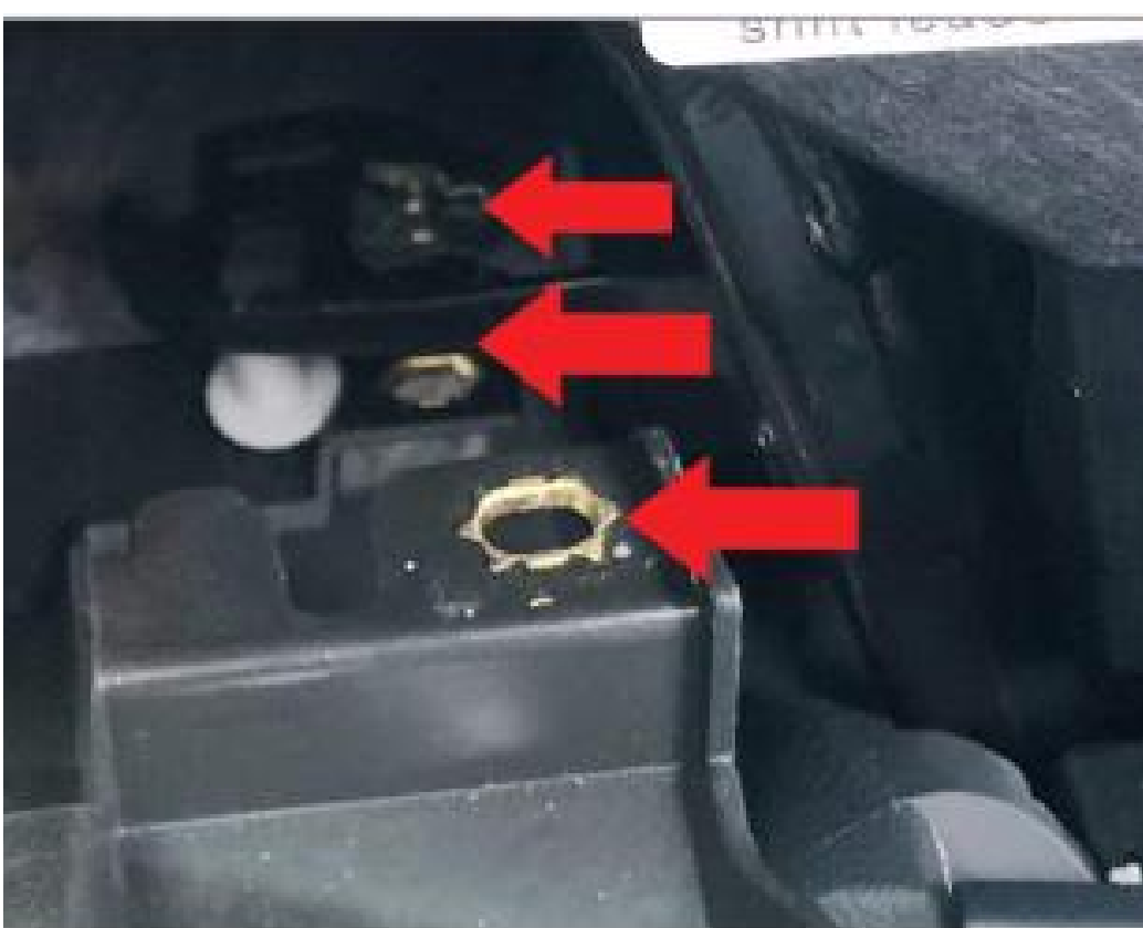
21. Place the new lower screen trim supplied (reuse the factory metal clips for the trim).
