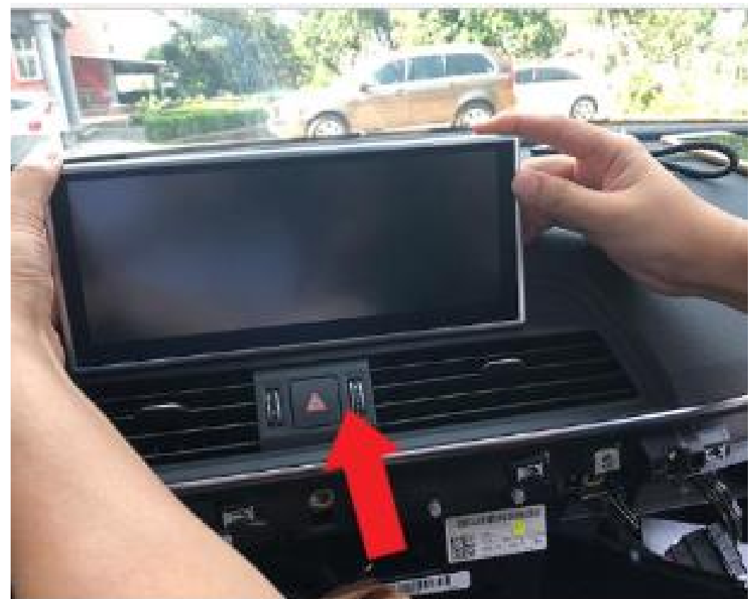
20. Carefully lift up the screen. Do not try to remove the screen completely as it is not designed to be removable.
