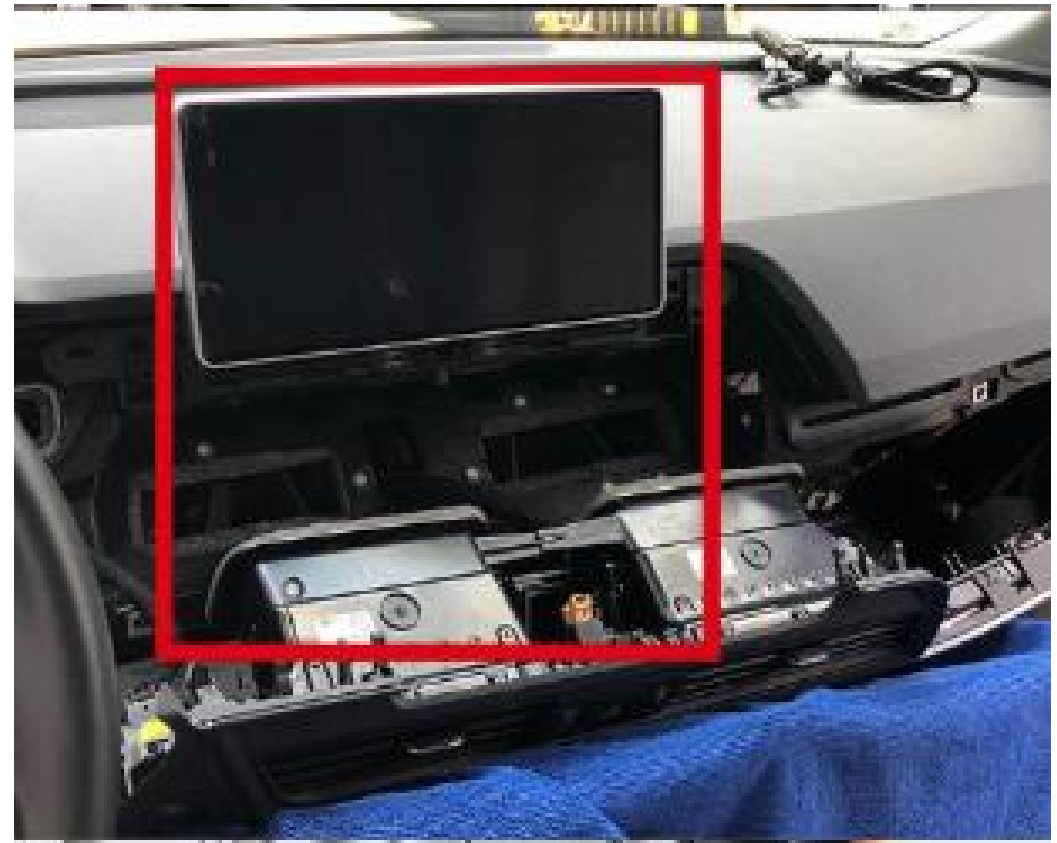
14. Place a large towel under the removed frame and disconnect necessary connectors.
