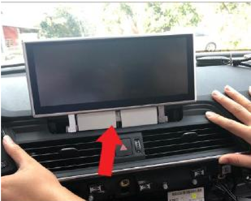
21. Place the new lower screen trim supplied (reuse the factory metal clips for the trim).
