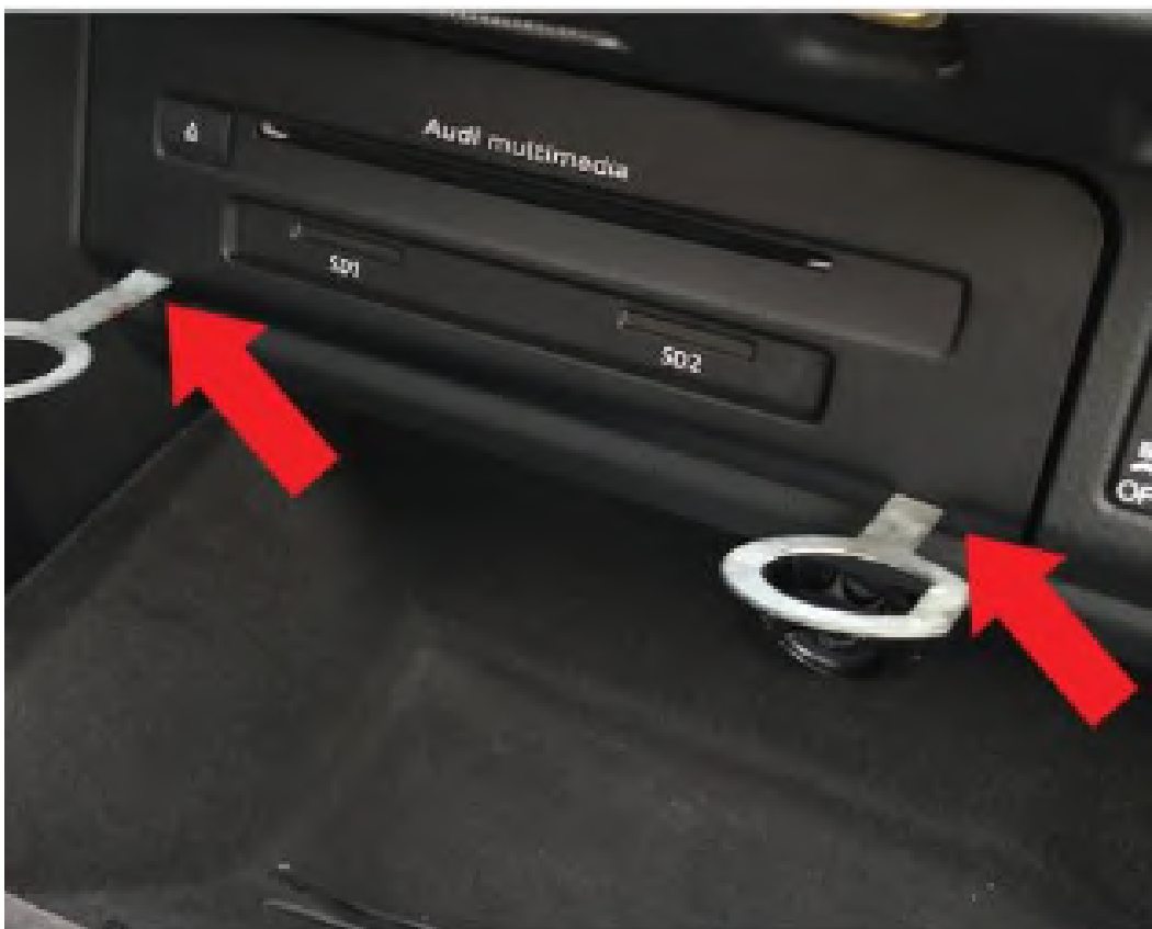
9. Remove the MMI head unit using a VAG Radio removal tool.
