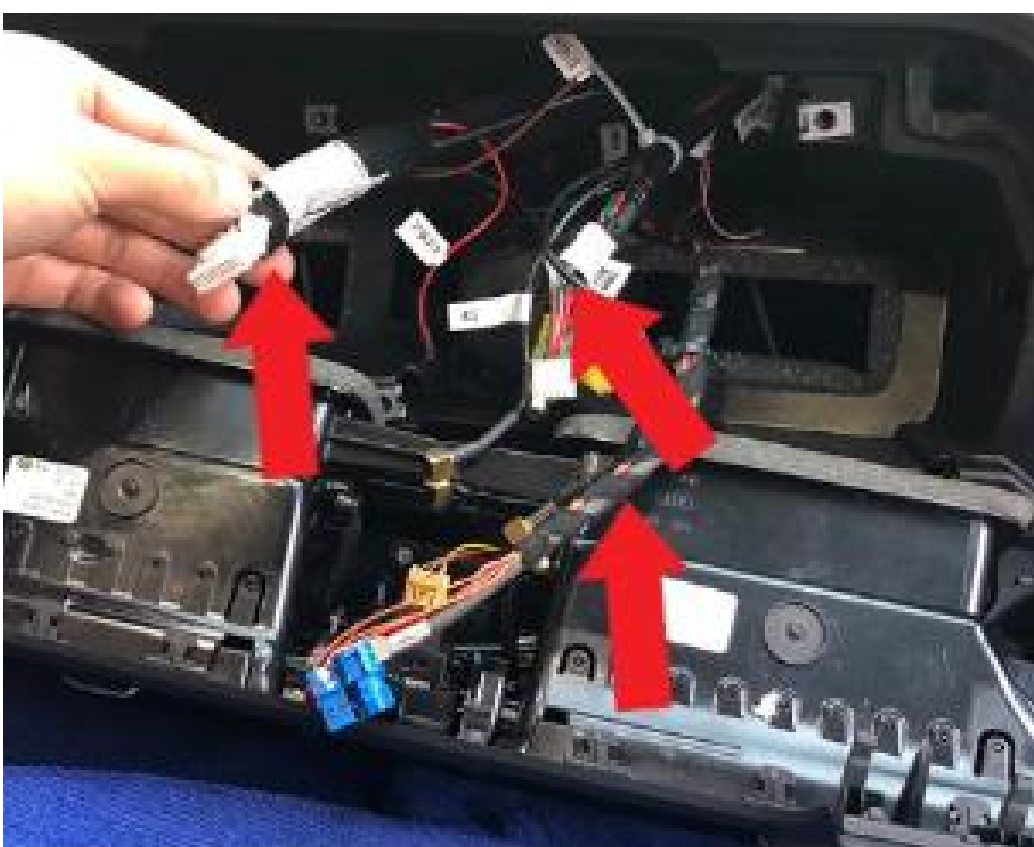
17. Route the cable into the screen opening by passing it behind the air ducts from the glove box.
