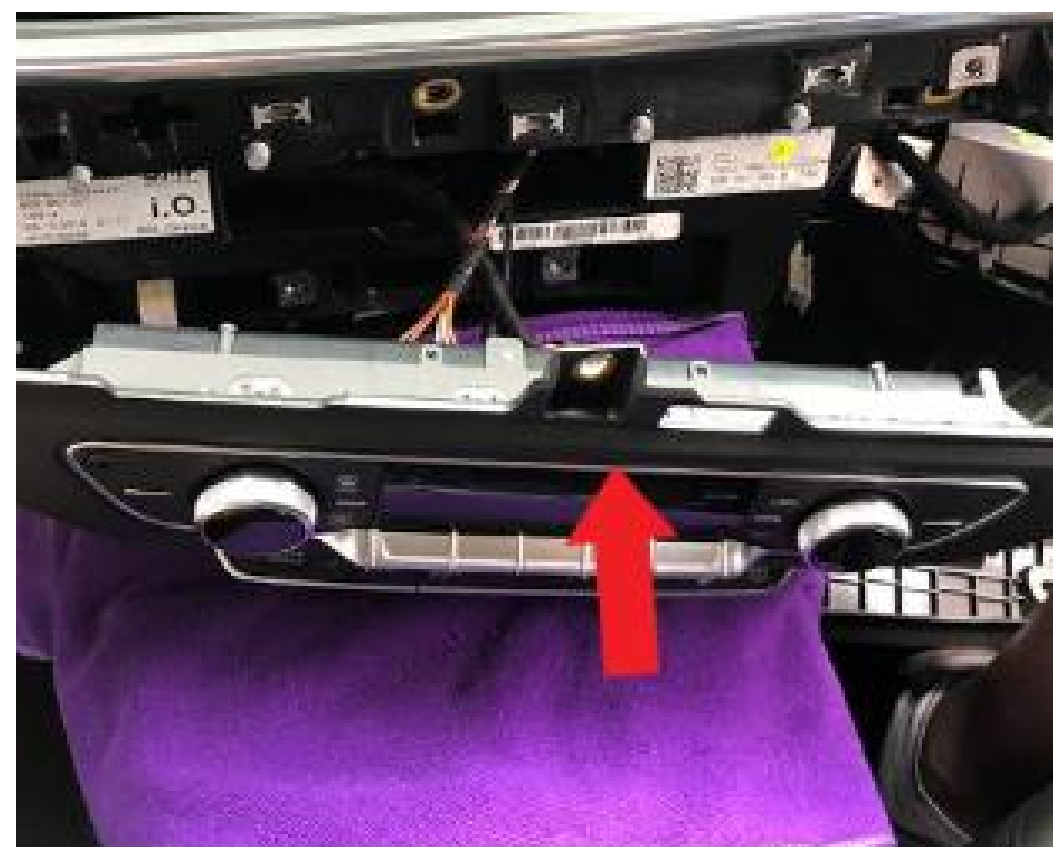
12. Unscrew the upper screw holding the center dash climate control panel trim and carefully remove the trim.
