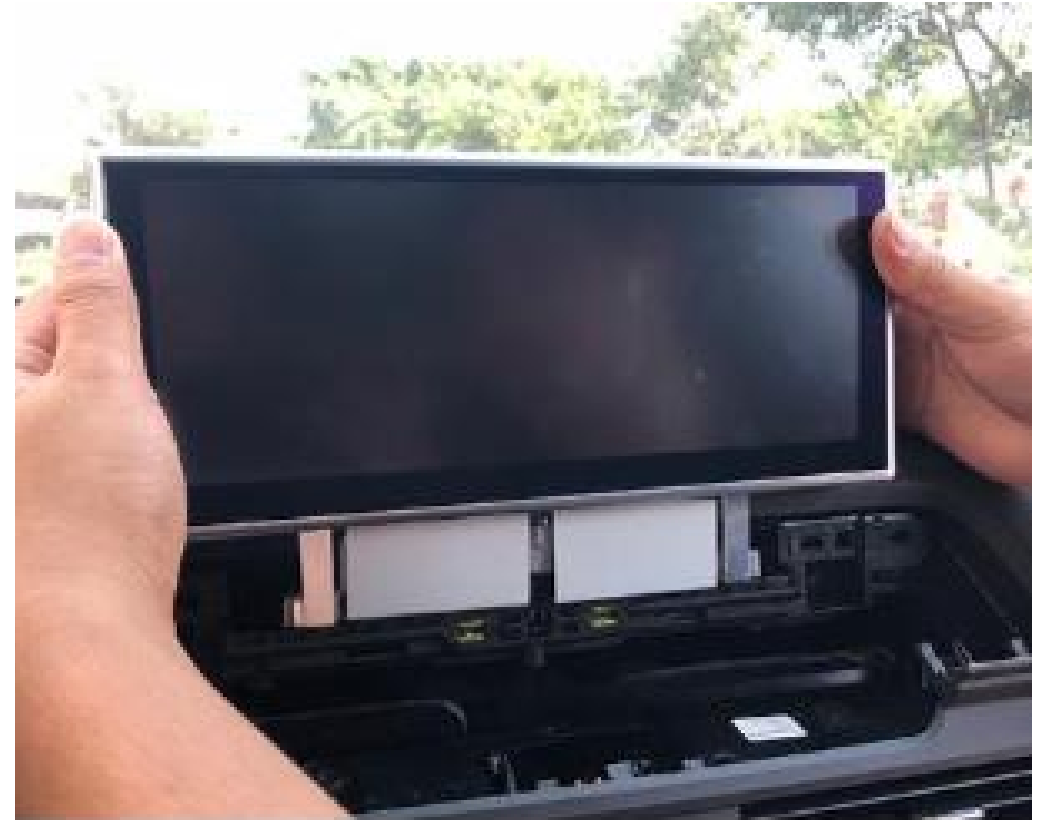
20. Carefully lift up the screen. Do not try to remove the screen completely as it is not designed to be removable.
