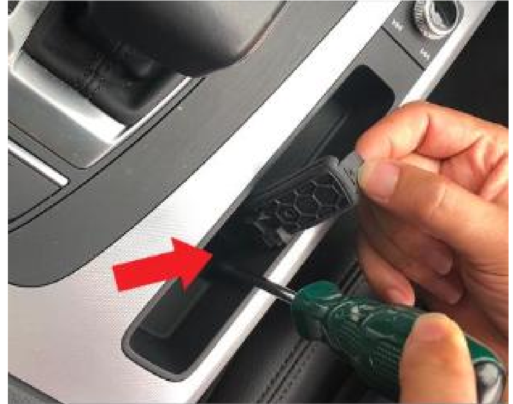
2. Unscrew the gear selector trim holding screw located under the coin tray.
