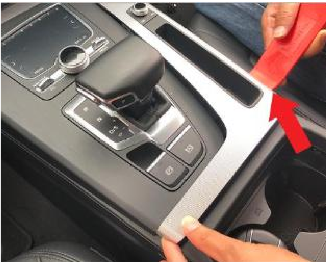
3. Carefully pry up the trim and remove it.
