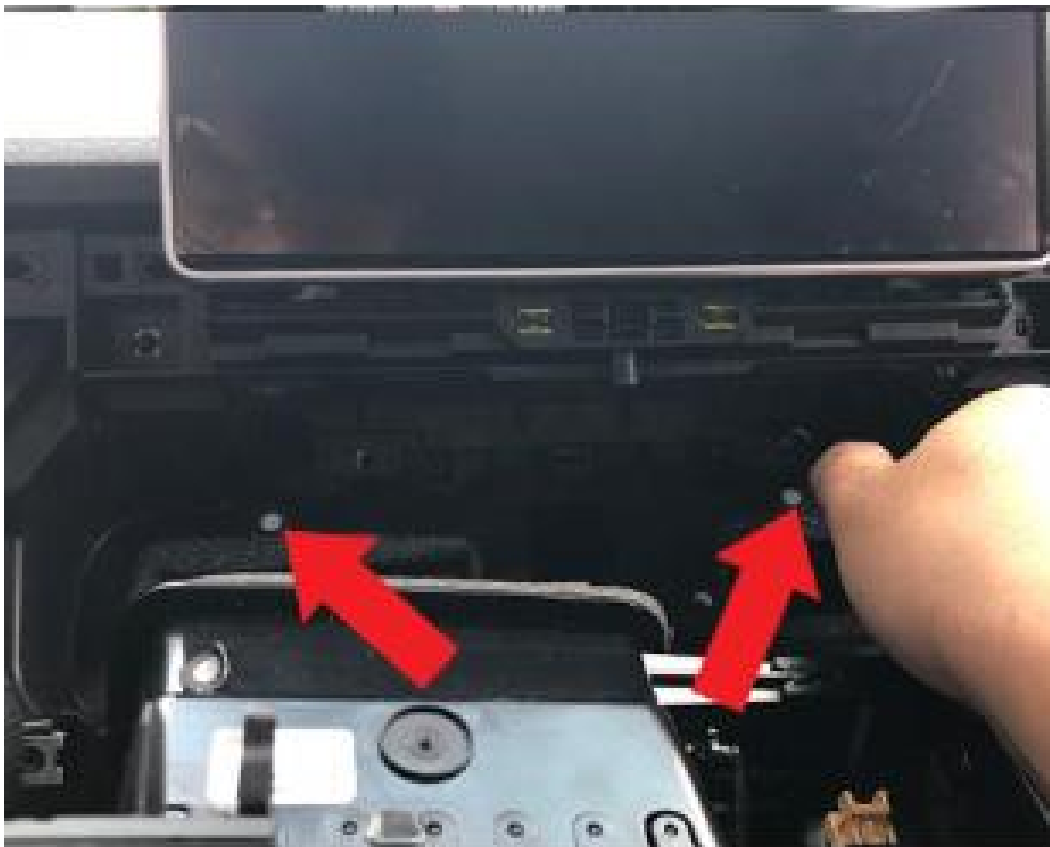
15. Remove the four screws holding the original screen.
