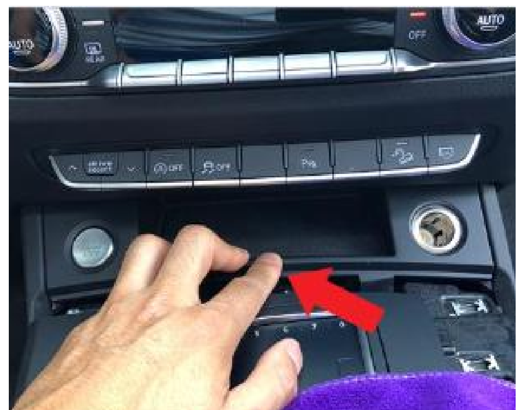
24. After properly installing the climate control trim, proceed to reassemble everything starting with the installation of the start button panel.
