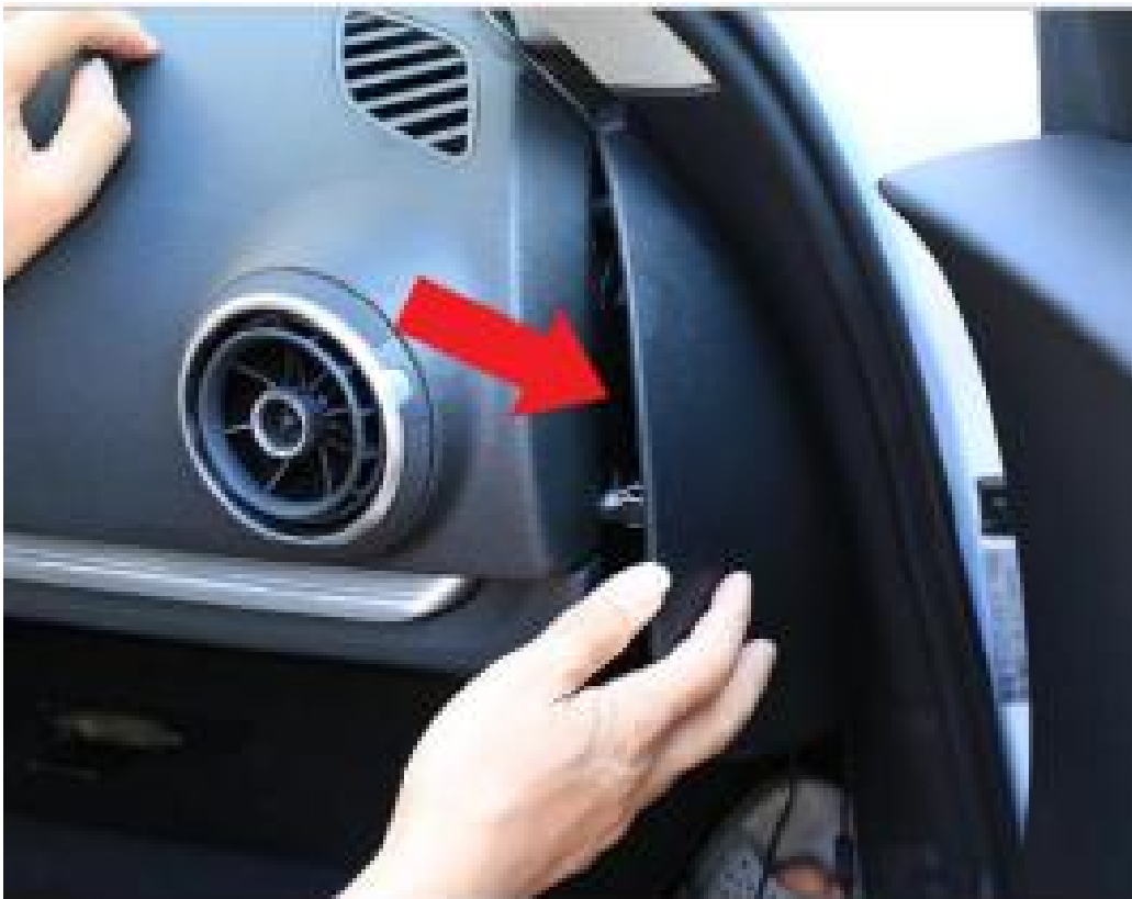
7. Remove the passenger side fuse panel cover.
