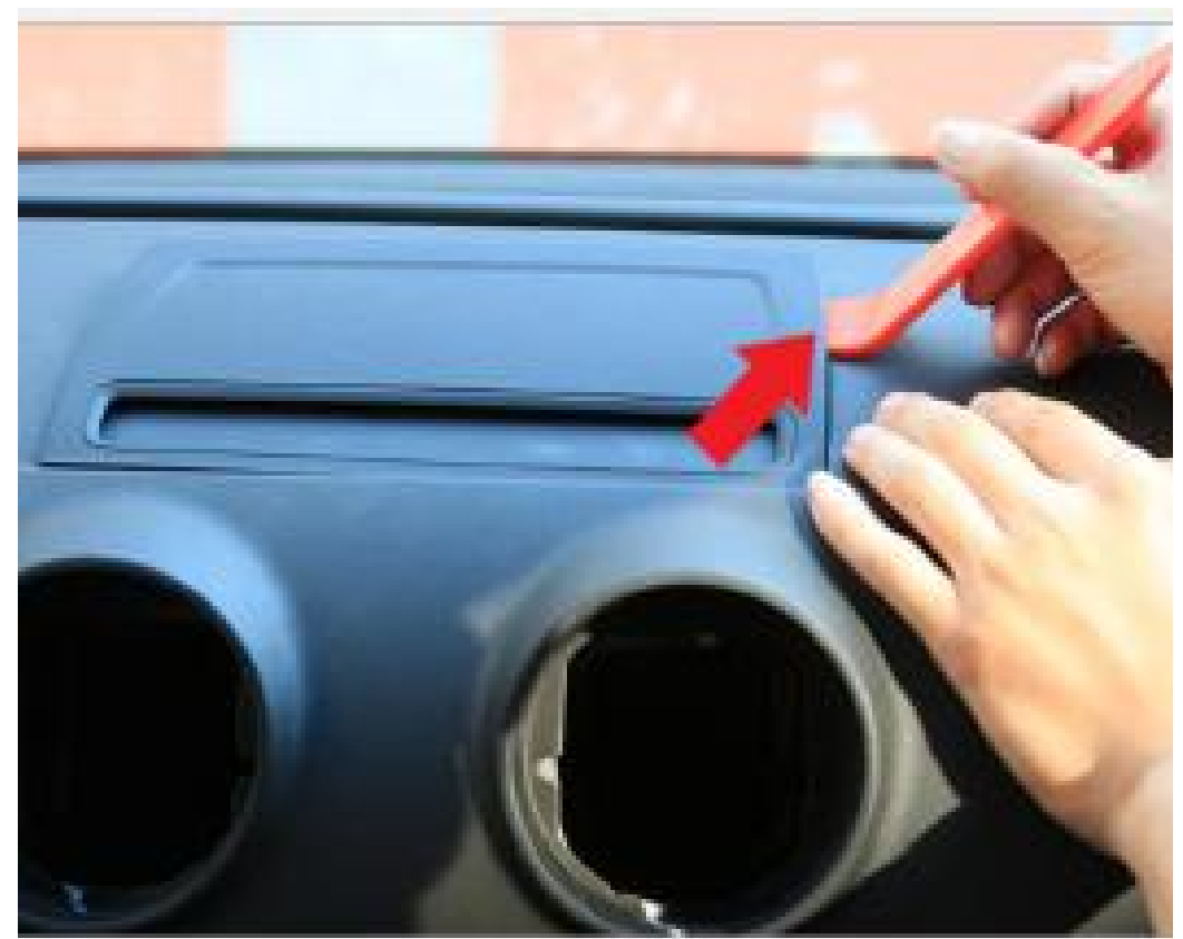
4. Pry up the screen cover trim and remove it.
