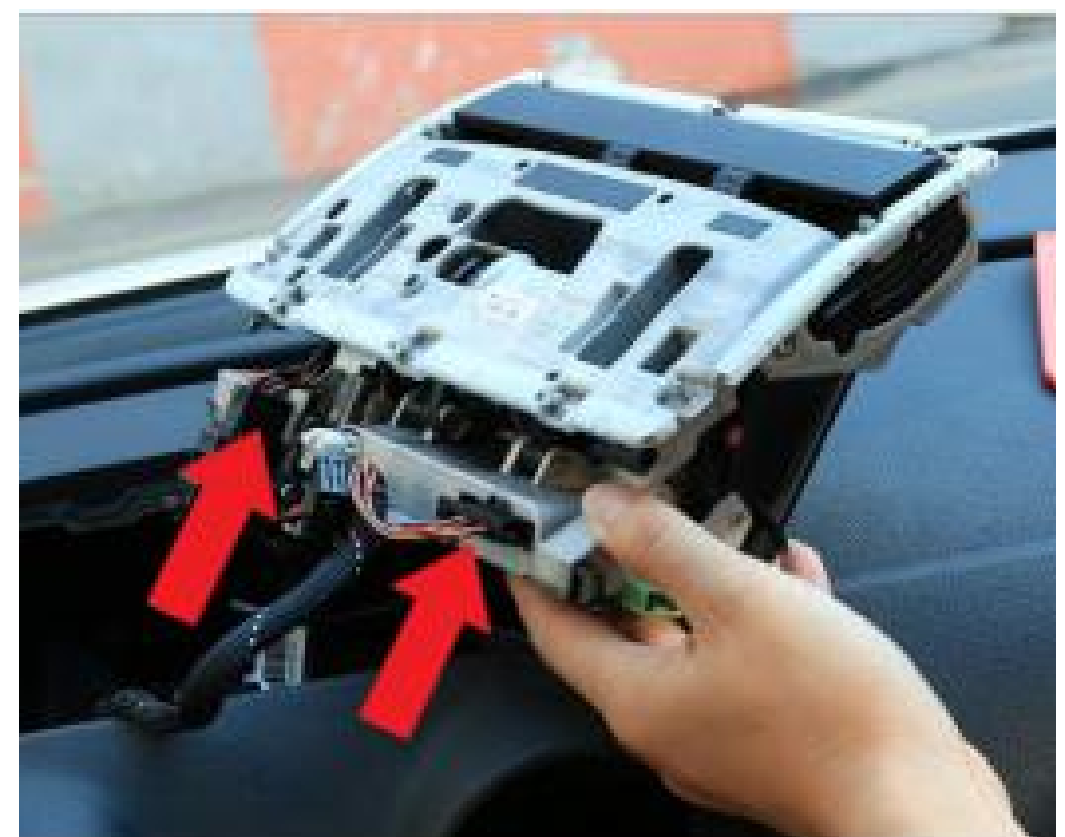
6. Remove the screen mechanism by disconnecting the LVDS and motor mechanism connector.
