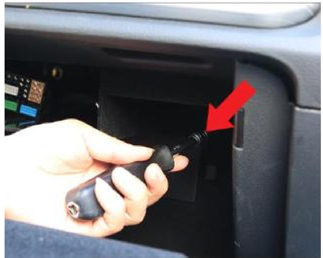
10. Remove the screw on the right side as well.
