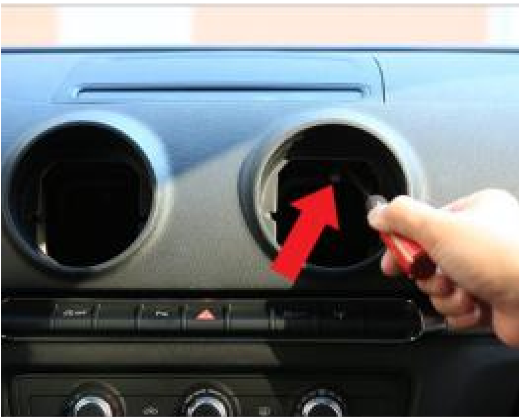
3. Unscrew the screen mechanism holding screws, one at each hole.
