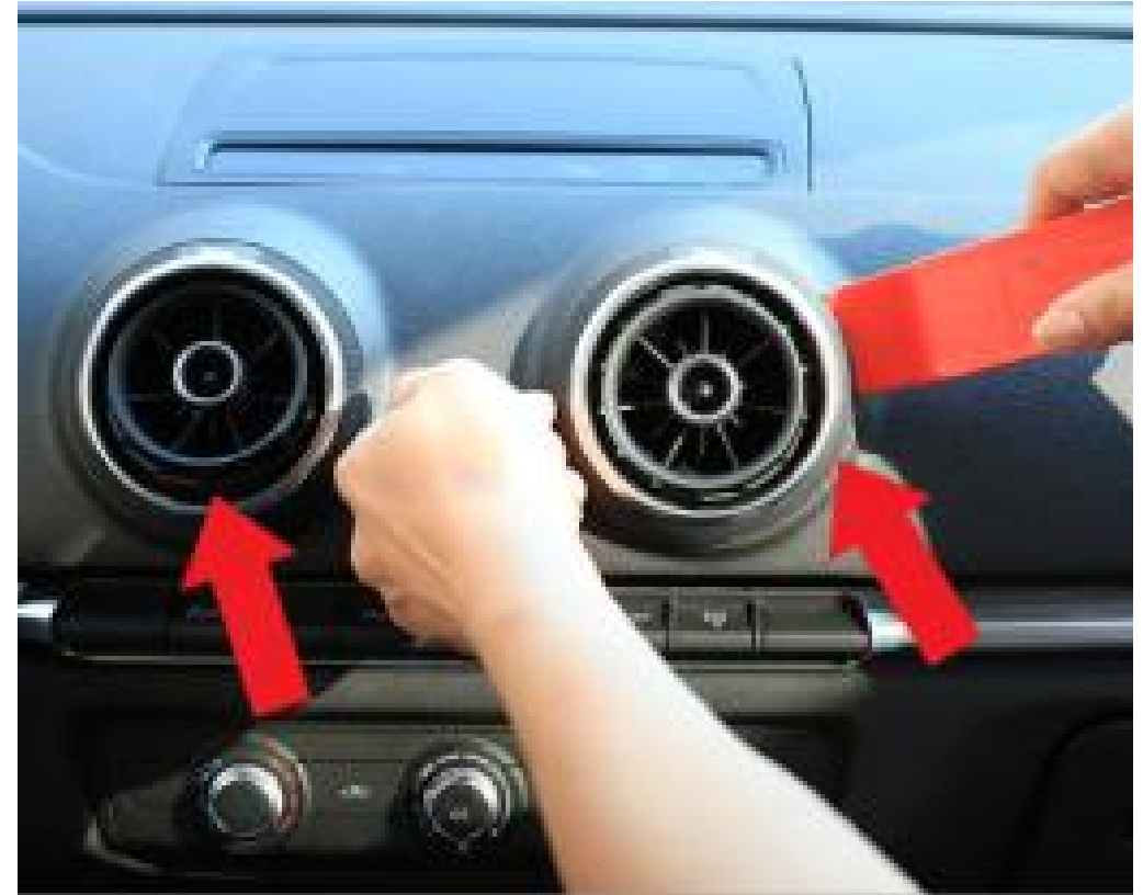
2. Using a prying tool, remove the center air vents.
