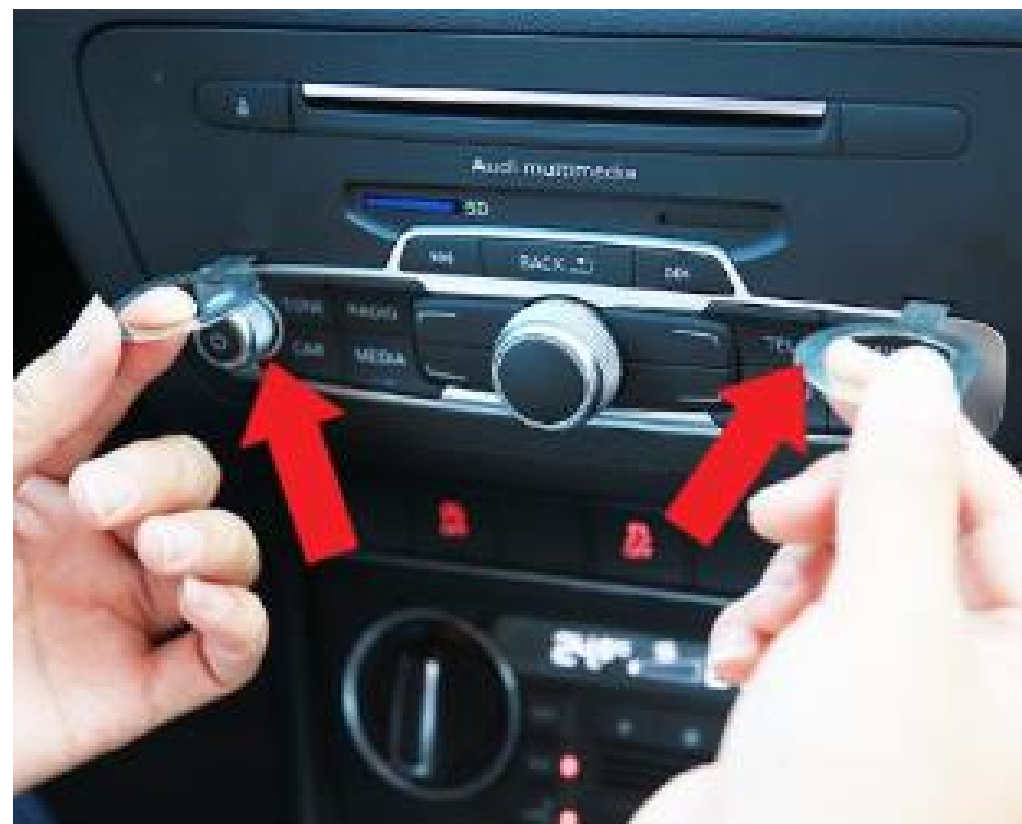
2. Use VAG Radio removal keys to remove the Radio/MMI head unit.
