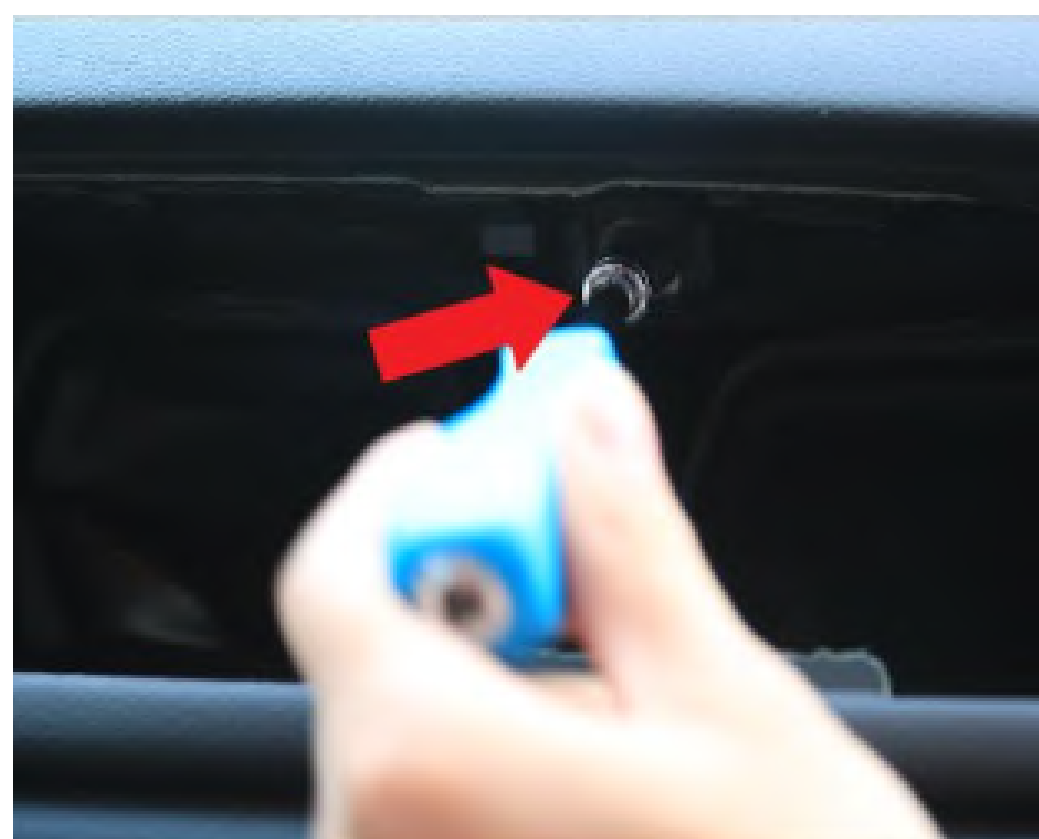
6. Unscrew the 8mm hex screw holding the screen.
