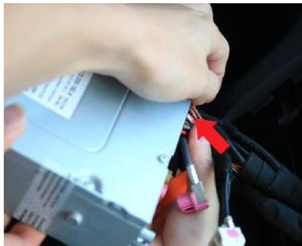
4. Unplug all the connectors behind the radio/MMI.
